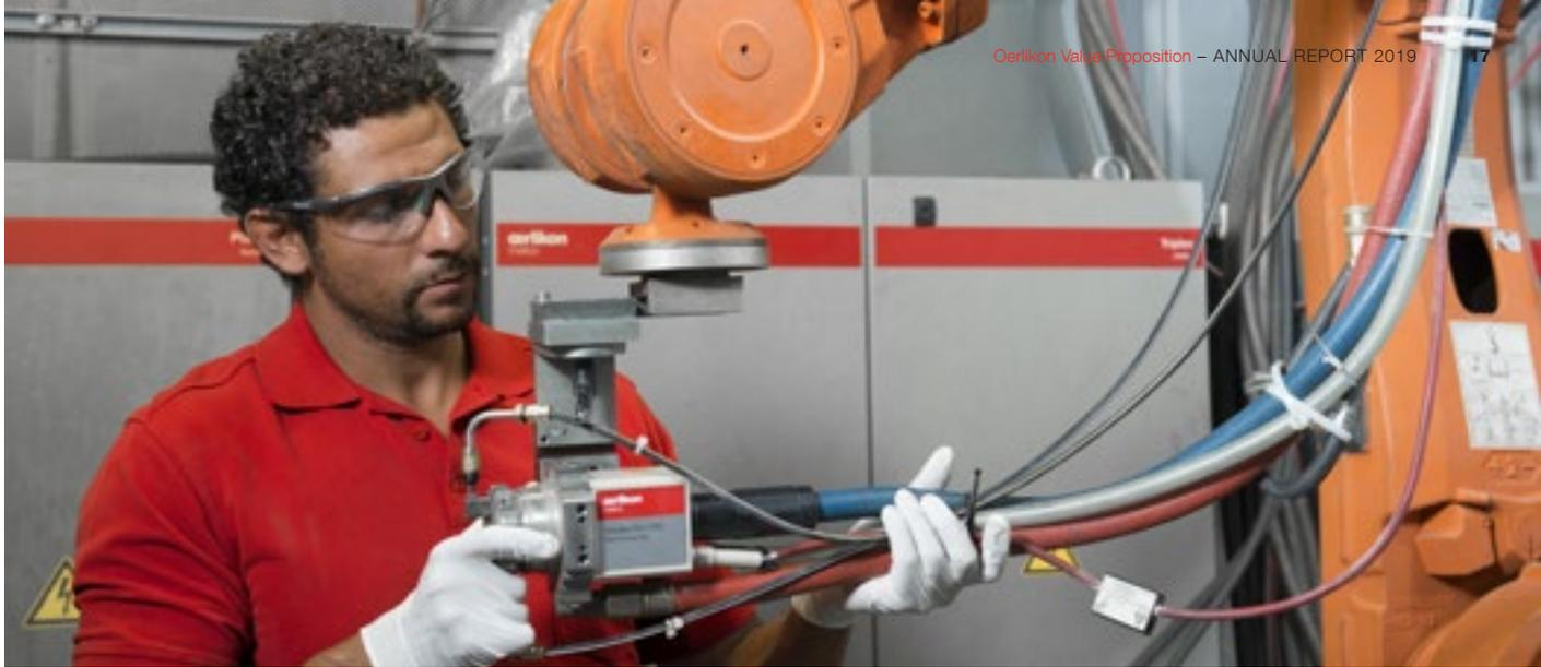
Oerlikon Metco's plasma spray guns are configured exactly according to customer needs for thermal spray coatings.
