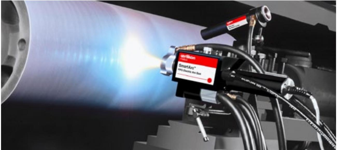
Oerlikon Metco's push pull gun (PPG) electric arc wire spray guns offer a high degree of flexibility and reliability to deposit hard and soft functional coatings.
