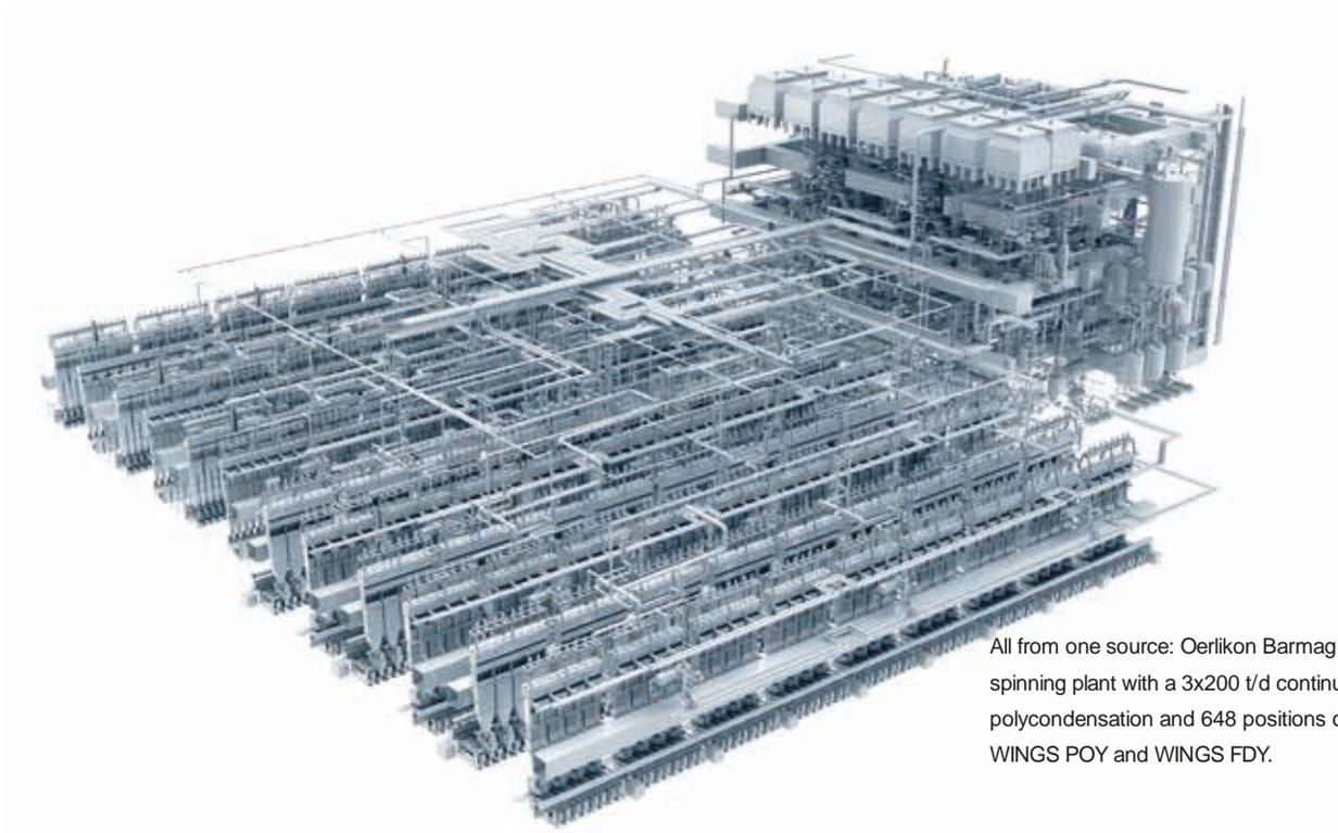
All from one source: Oerlikon Barmag spinning plant with a 3x200 t/d continuous polycondensation and 648 positions of WINGS POY and WINGS FDY.
