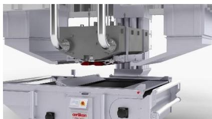
**Caption 1:** The hycuTEC process easily achieves filtration efficiencies in excess of 99.99% in the case of typical filter media.
