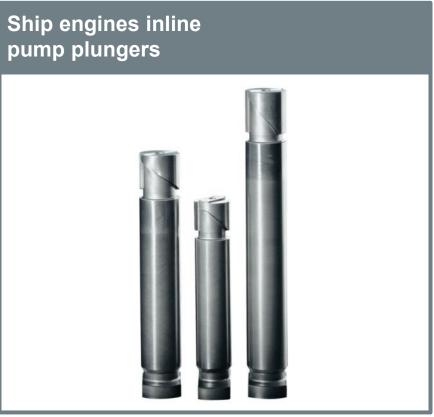
Injection pressures of advanced diesel injection systems reach today more than 2000 bar. This results in seizure of µm tolerated plunger, rings or discs BALINIT® C (WC/C) of plungers for large ship pumps or BALINIT® DLC of common rail pumps are today a design standard.
