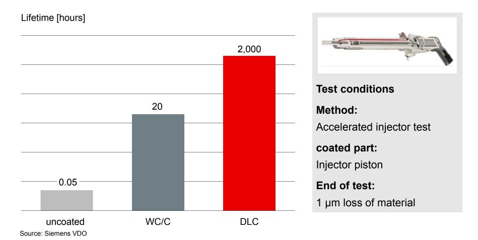
Increasing injection pressures lead to severe seizure problems on diesel injector components. BALINIT® DLC achieves the highest wear resistance for injector components.
