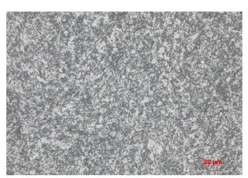
Martensitic, iron-chromium, air-hardenable steel powder products with chemistries similar to AMS 6408, AISI H13, ASTM H13, SAE H-13 and Werkstoff No. 1.2344 / X40CrMoV 5-1-1. Room temperature static properties of LB-PBF processed and heat treated material coupons have been shown to be comparable to those of AMS 6408.
