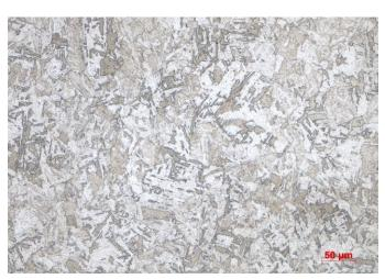
A family of martensitic, precipitation-hardening stainless steel alloy products with chemistry similar to AMS 5659. Room temperature static properties of LB-PBF processed and heat treated material coupons have been shown to be comparable to those of AMS 5659 in the H900 state.
