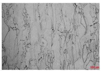
A family of nickel-based solid solution strengthened powder products with chemistry similar to AMS 5536, EN 2.4665 and UNS N06002. This material has been optimized to mitigate cracking when processing with Laser Powder Bed Fusion (LPBF).
