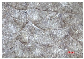
A FeNiCo-based powder similar to 18 Ni maraging steel (M300 type). The chemical composition is similar to that of AMS 6514, Werkstoff Nr. 1.2709 / X3NiCoMoTi 18-9-5 and UNS K93120. The material is optimized for producing additive manufactured components using Laser Powder Bed Fusion (LB-PBF).
