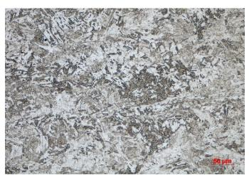
A family of martensitic, precipitation-hardening stainless steel powders with chemistry similar to AMS 5643. Room temperature static properties of LB-PBF processed and heat treated material coupons have been shown to be comparable to those of AMS 5643 in the H900 state.
