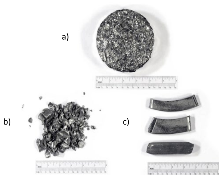
Fig. 1 Variations in titanium scrap feedstock for ISM: (a) turnings compacted into 'briquettes', (b) cobbles and (c) solids [1]
