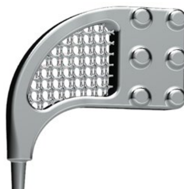
An example lattice structure created using the NX Lattice Structures Design module (Courtesy Siemens)
