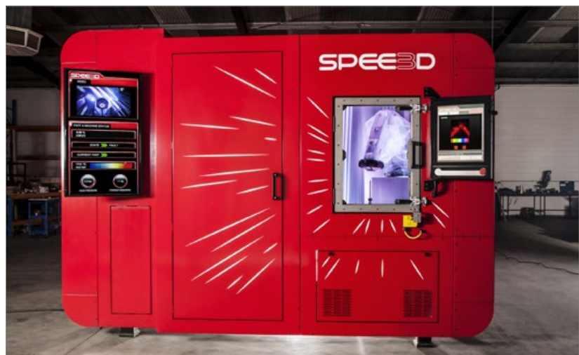
SPEE3D utilises a high speed six axis robot in its metal AM system
