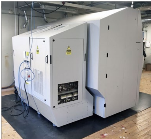
Fig. 5 A steel plate was used to spread the weight of this machine when it was discovered that the floor was not strong enough (Courtesy Olaf Diegel)
