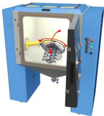
Solukon systems automate the cleaning of metal parts
