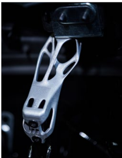
The part is used to carry a cover which unfolds when opening the roof
