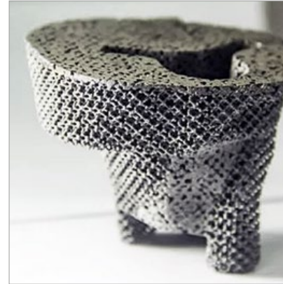
An AM tantalum implant was used to fill defects in an 84 year old man's knee (Courtesy China Global Television Network)
