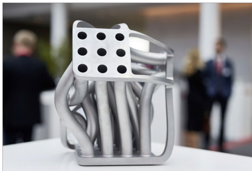
Fig. 1 An additively manufactured AlSi10Mg distributor housing produced by Oerlikon's AM facility in Barleben, Germany
