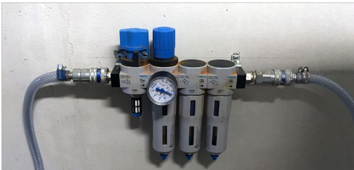
Fig. 6 An air filter may be required to safely operate a metal PBF system (Courtesy Olaf Diegel)
