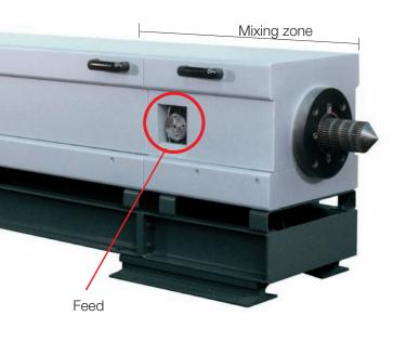
The mixer unit is attached to Oerlikon Barmag extruders as a screw and barrel extension. The masterbatch to be added is introduced into the mixing zone either via the extruder hopper (granulate/liquid additive) or through the side (melted or in liquid form). The mixing zone can be heated and cooled separately.
