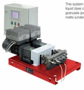
This system was developed for feeding liquid dyes or additives into plastic granulate (pressureless) or in polymer melts (under pressure).
