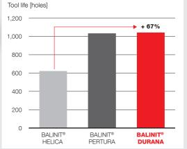
Solid carbide drill Ø 8.5 mm Steel 1.7225 42CrMo4 (AISI4140, SCM440) Cutting data  $v_{c} = 160 \text{ m/min}$ f = 0.26 mm/rev
