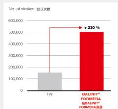
Tool Extrusion die ② 60 mm, 5 station cold former Collar nut manufacturing 直径60mm的挤压模,5工位冷成型螺母制造
