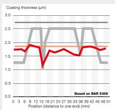
MoN coated piston pin after 500h engine test:
