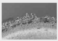
Surface fatigue detail of a valve plate (100x).
