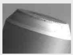
Fine abrasion and micro fatigue of a valve stem (10x).
