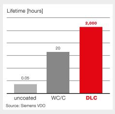
Comparative result of uncoated injector needles versus those coated with BALINIT® C or BALINIT® DLC showing the advantage of the harder DLC coating during high-load injector testing.
