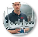
Clean surfaces are essential for coating adhesion. So Oerlikon Balzers invests a great deal of effort in surface preparation for PVD and offers multi-stage ultrasonic cleaning lines using aqueous alkaline baths with no environmentally harmful additives.
