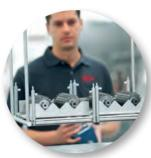
Clean surfaces are essential for coating adhesion. So Oerlikon Balzers invests a great deal of effort in surface preparation for PVD and offers multi-stage ultrasonic cleaning lines using aqueous alkaline baths with no environmentally harmful additives. 清洁的表面对于涂层的附着力至关重要。因此,欧瑞康巴尔查斯为PVD的表面准备方面投入了大量精力,并提供碱性水溶液的多级超声波清洗线,不含对环境有害的添加剂。
