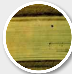
Wear track (30x) of BALINIT® C coated ring exhibits only slight running in (wear depth approx 0.2 \mu\text{m} ) after 2000 m sliding distance
