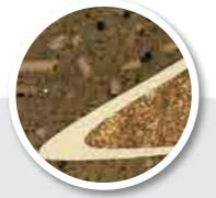
BALINIT® coatings have thicknesses measured in micrometers, preserving blade precision and sharpness.
