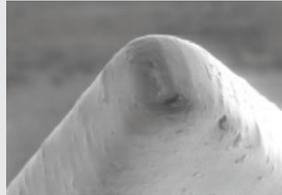
Nearly no wear of BALINIT® CNI coated dents of opening cylinder after 3000 hours polymer spinning.
