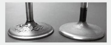
BALINIT® FUTURA NANO prevents hydrocarbon buildup on valves.
