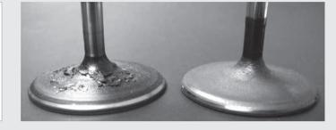
BALINIT<sup>®</sup> FUTURA NANO prevents hydrocarbon buildup on valves.
