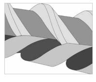
BALINIT<sup>®</sup> DLC for screw spindles shows significantly longer lifetime compared to nitride steel DIN 1.7131 in abrasive grinding cooling media.
