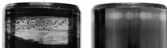
Positive effects of BALINIT® DLC coated wrist pins.
