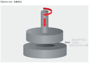
Effect of BALINIT® DLC coating on the weight loss of a thrust washer test - coated verse uncoated washers (bottom washer coated, total wear of both washers).
