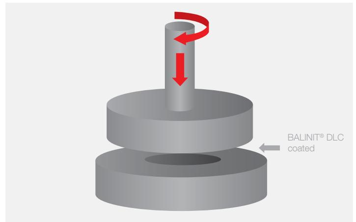
Effect of BALINIT® DLC coating on the weight loss of a thrust washer test – coated verse uncoated washers (bottom washer coated, total wear of both washers).
