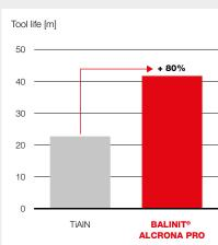
Wet machining of carbon steel
