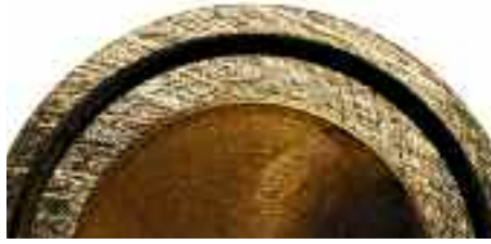
Bronze: abrasive wear and deformation
