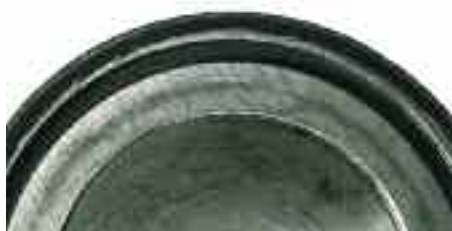
Steel and BALINIT® C (WC/C): wear < 1 µm
