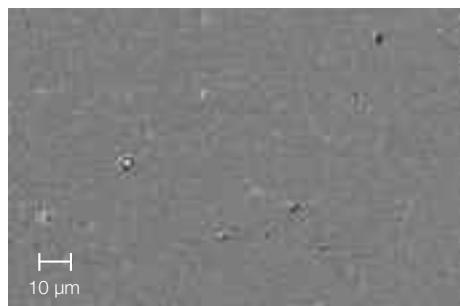
Surface of a PVD arc coating after finishing
