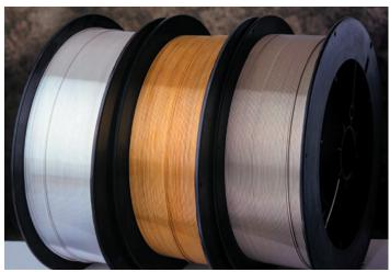
ated rate if kept in a warm, humid atmosphere. Most of these types of materials will be slightly lubricated not only to improve wire feeding, but also to reduce this corrosion effect. Care must be taken not to remove the lubricant film during storage.
