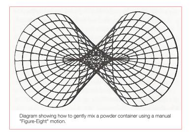
the bottom of the container. For blended materials such as Metco 601NS and Metco 81VF-NS, the lower density phase can separate out towards the top of the container. In all cases, this means that best practice is to gently tumble the powder before spraying. This ensures uniform product distribution and uniform coating results.
