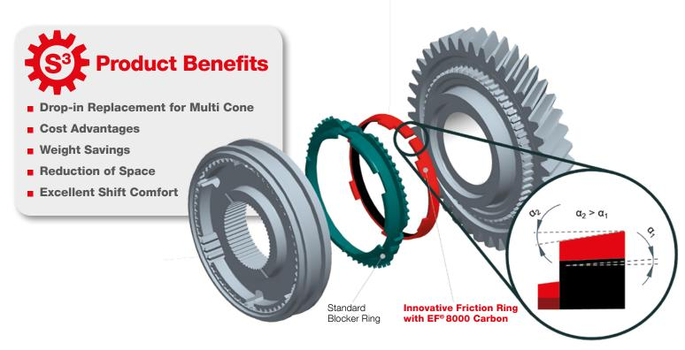
The innovative Segmented Synchronizer System S³ provides weight, space and cost benefits compared to conventional multi cone synchronizers while maintaining equivalent per-formance and shift quality. The key innovation is a split friction ring with a small inner cone angle for generating high friction torque and a large outer cone angle for release without self-locking.
