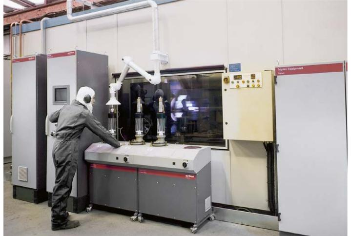
Coating applications engineer monitors the application of a Metco PUMP coating to vital pump parts, such as impellers, casings and wear rings.
