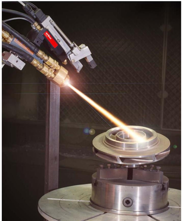
Laboratory and field tests have proven that Metco PUMP coatings, developed for pump components subject to severe abrasion, significantly increase service life.
