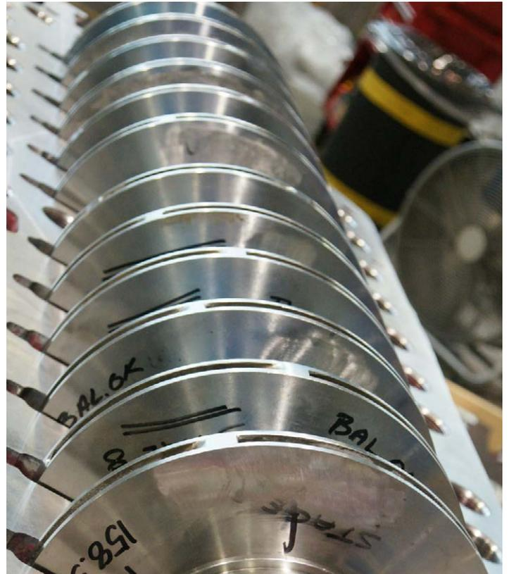
The impeller blades and the shaft of a large centrifugal seawater injection pump. Areas of pump that will be subjected to erosive and corrosive action of seawater loaded with abrasive particles have been thermal spray coated with Metco PUMP long-life coatings.
