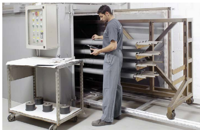
Cross-linking of polymer via post-coat heat treatment
