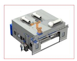
An innovative thermal spray installation for coating large, heavy industrial rollers that features four processes in one system: atmospheric plasma spray, liquid-fuel HVOF, electric arc wire and post-coat sealing.
