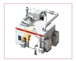
In conventional spraying, the bulky transition duct is rotated or indexed while the plasma gun is moved axially through the transition duct. Our more efficient solution rotates the plasma spray gun while keeping the workpiece stationary.
