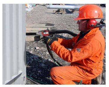
Coating a container with a zinc-aluminum coating
