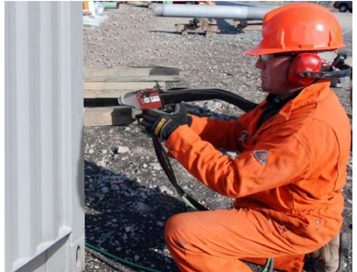
Coating a container with a zinc-aluminum coating
