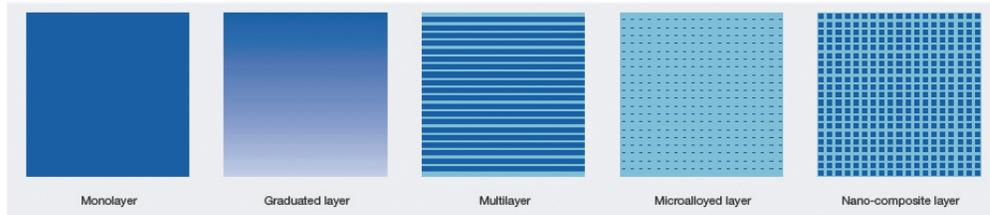
Functional coating properties, such as the layer hardness, the phase stability, and the tribological properties, can be adjusted by a different distribution of the elements within the layer
