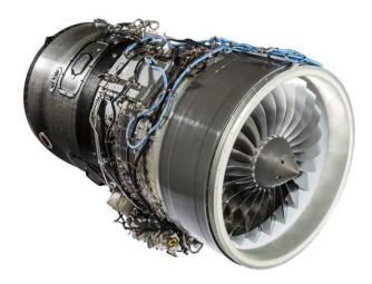
Oerlikon Balzers signed a ten-year contract with ITP Aero to use its new high-temperature wear resistant coating on ITP Aero's next generation aero engine components of the Pratt & Whitney Canada PW800 turbofan engine that powers the new Gulfstream G500/G600 business jets. (© copyright: Pratt & Whitney)
