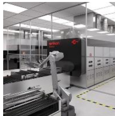
The INUBIA I6 system provides chrome-looking plastic metallisation using Oerlikon Balzers' ePD technology.
