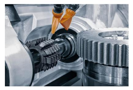
BALINIT ALCRONA EVO has already demonstrated its capabilities in a test conducted by a Tier 1 automotive supplier for gear hobbing, increasing tool service life by more than 40 percent. Image: AdobeStock
