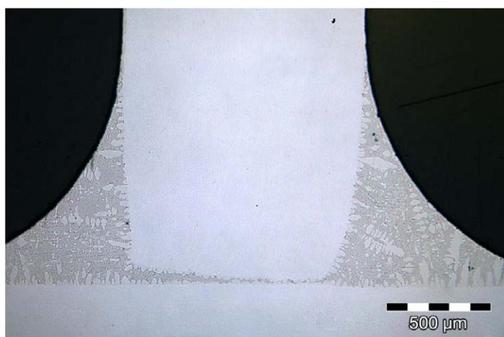
A T-joint brazed with AMDRY 105 demonstrates its ability to fill small gaps while maintaining good fillet characteristics.
