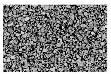
SEM photomicrograph showing the typical morphology of Metco 6485
