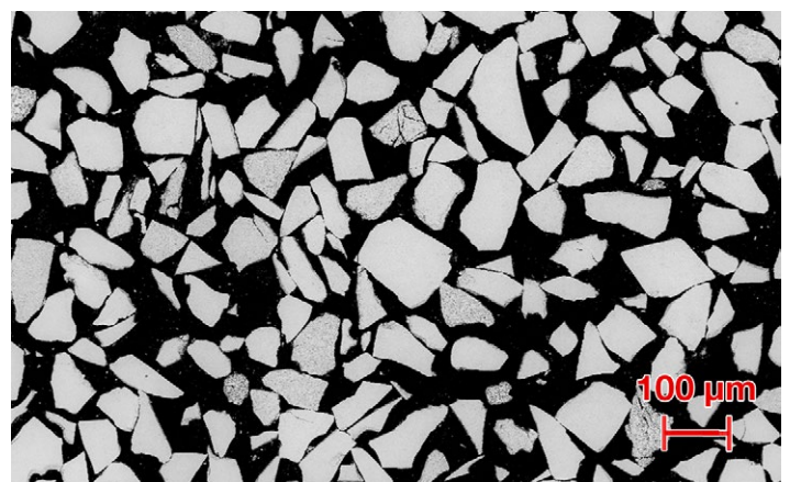
Typical SEM photomicrographs. Top: exterior blocky / irregular morphology. Bottom: fully dense interior structure.
