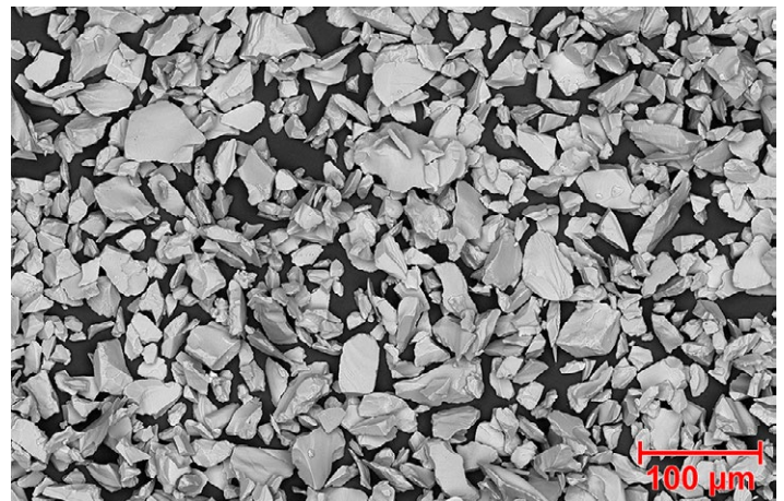
SEM Photomicrograph of Metco 102 showing typical fused and crushed morphology of these materials.
