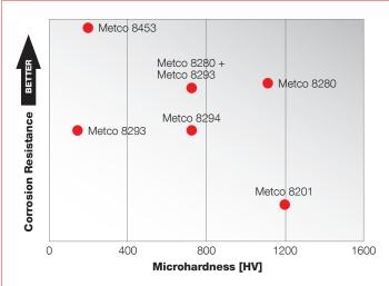
Corrosion and hardness comparison for electric arc wire coating materials
