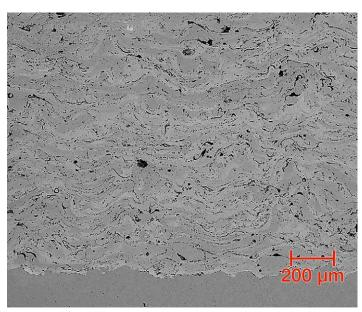
Typical as-sprayed coating microstructure of Metco 8280.
