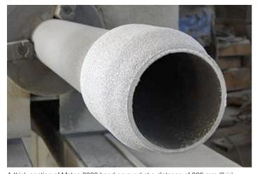
A thick coating of Metco 8280 hand-sprayed at a distance of 200 mm (8 in). Notice the light gray, metallic appearance of the coating. This is indicative of the low oxide microstructure of Metco 8280, which results in high bond strength and consistent coating quality.
