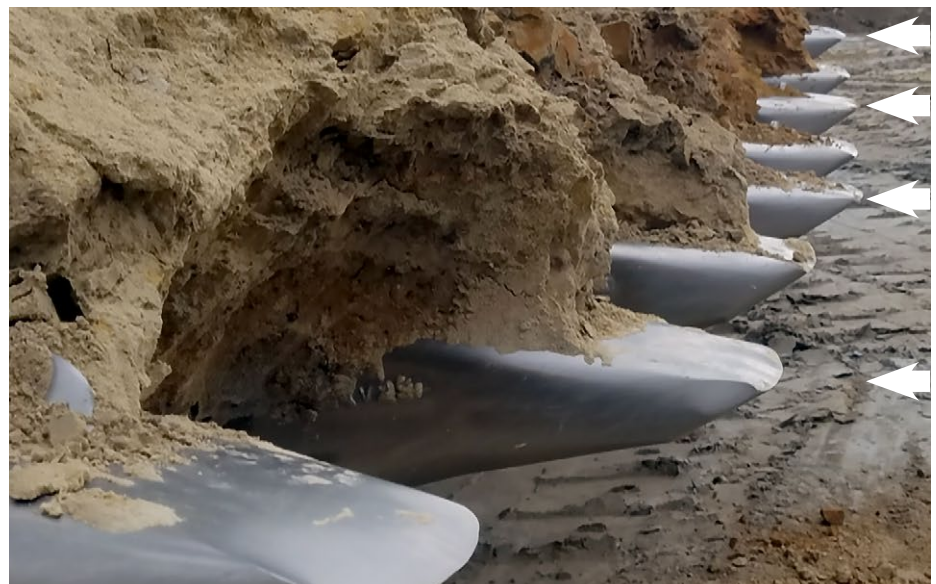
Trials using Metco 8247, on GETs in service. ( left ): Close-up of hardfaced GET. ( right ): Comparison of hardfaced and unhardfaced GETs. White arrows highlight the hardfaced GETs. Notice that the hardfaced GETs are longer and less worn, attesting to the abrasion resistance of Metco 8247.
