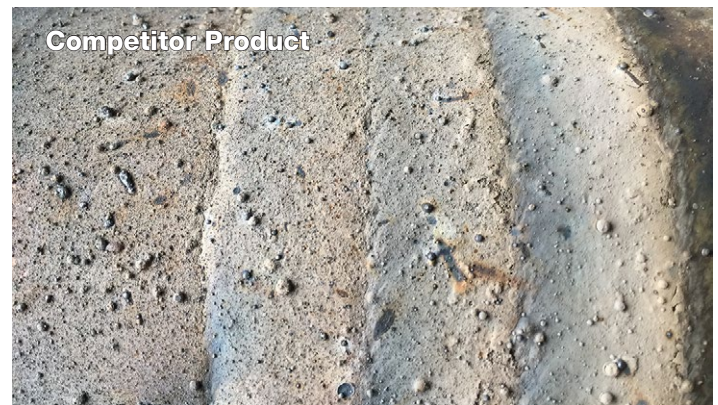
Weldability is improved with Metco 8247 ( left ) compared to competitive hardbanding materials ( right ). The cleaner, low spatter weld generated using welding Metco 8247 lowers both the post-weld grinding time and the potential for sub-surface porosity. The smoke-free weld deposition of Metco 8247 improves operator safety and allows the operator to better control the quality of the weld.
