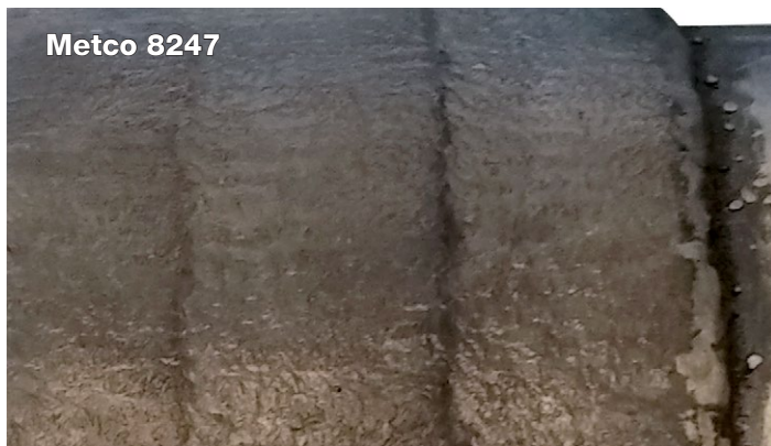
Weldability is improved with Metco 8247 ( left ) compared to competitive hardbanding materials ( right ). The cleaner, low spatter weld generated using welding Metco 8247 lowers both the post-weld grinding time and the potential for sub-surface porosity. The smoke-free weld deposition of Metco 8247 improves operator safety and allows the operator to better control the quality of the weld.
