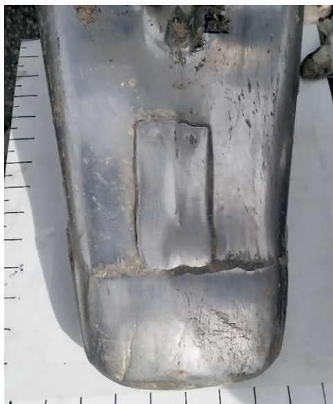
Trials using Metco 8247, on GETs in service. ( left ): Close-up of hardfaced GET. ( right ): Comparison of hardfaced and unhardfaced GETs. White arrows highlight the hardfaced GETs. Notice that the hardfaced GETs are longer and less worn, attesting to the abrasion resistance of Metco 8247.
