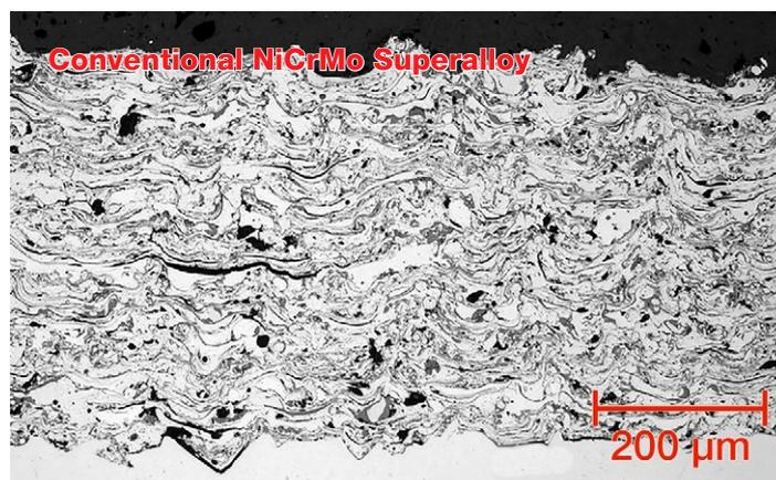
Metco 8453 (top) forms coatings with much lower oxide content than coatings of a conventional NiCrMo superalloy (bottom). In addition Metco 8453 splat interfaces are less contaminated with oxide layers and the coating splats are generally larger and more interconnected.
