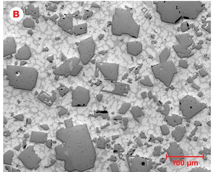
Microstructure comparison of Metco 8224 deposit **[A]** versus WC-Ni GMAW deposit **[B]**. Note the fine hard phase and more homogeneous structure created by Metco 8224 versus the very large hard phase particles in the WC-Ni GMAW deposit.
