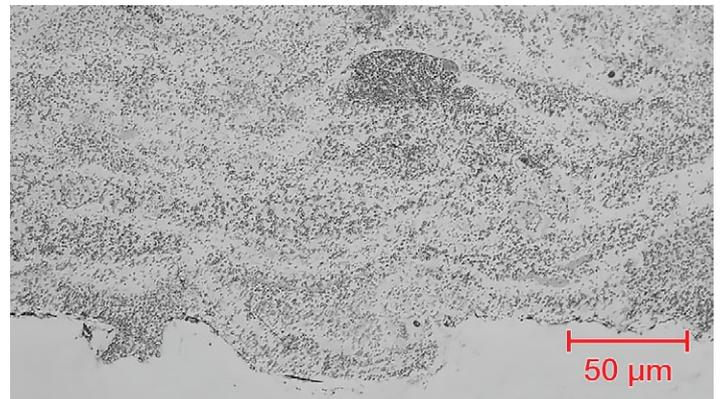
Top: Typical as-welded coating microstructure of Metco 1030x or Metco 8224.
