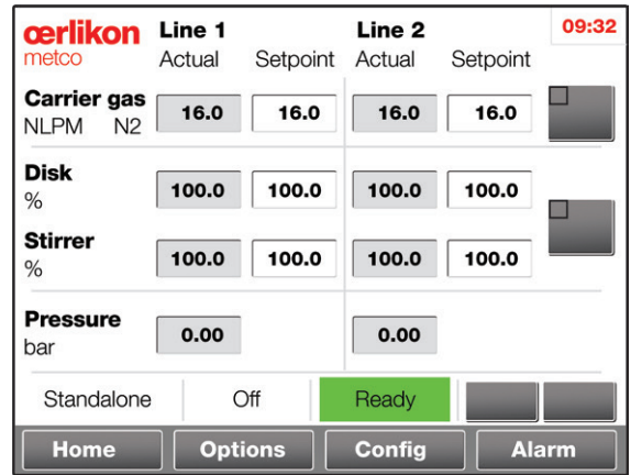
Touchscreen home page of the Metco Twin 150 Feeder
