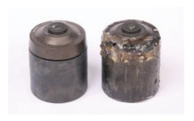
A spin pack assembled using lower quality components can result in leakages, downtimes and process variations.
