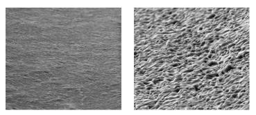
SEM RE of Oerlikon Barmag (left) and competitor ceramics images show the difference of the surface structure
