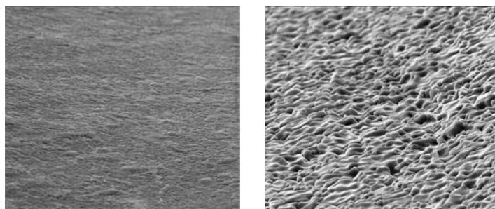
SEM RE of Oerlikon Barmag (left) and competitor ceramics images show the difference of the surface structure
