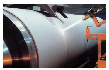
Figure 22 - HVOF coating of a sink roll
