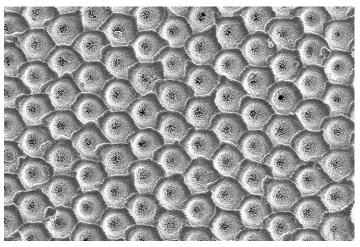
Figure 18 – Anilox printing roll with a laser engraved Metco<sup>™</sup>PRINT coating
