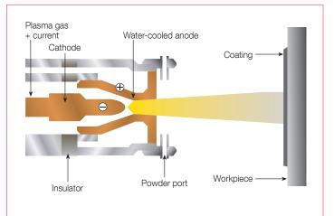
Figure 6a - Schematic diagram of the plasma spray process
