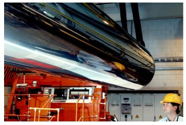
Figure 23 – Metco<sup>™</sup>CAL coating after superfinishing
