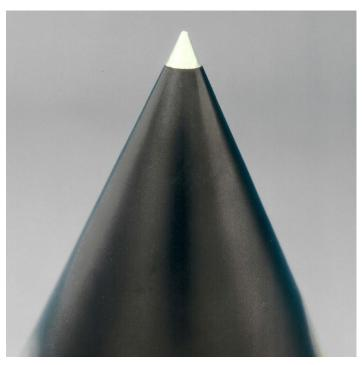
Figure 1b - Nozzle needle with a chrome oxide coating to prevent wear.
