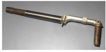
Figure 14 - Nose gear of an F5 Tiger with a WC/CoCr coating
