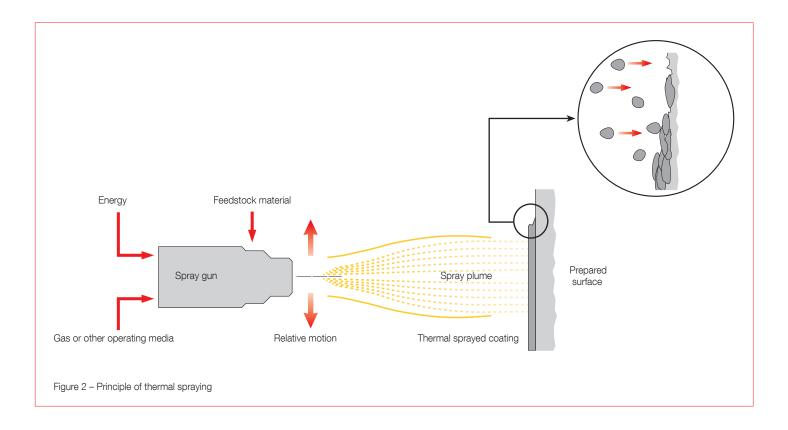
Heat from the hot particles is transferred to the cooler base material. As the particles shrink and solidify, they bond to the roughened base material. Adhesion of the coating is therefore based on mechanical "hooking". This procedure is represented schematically in Figures 2 and 3. The amount of metallurgical bond caused by diffusion between the coating particles and base material is small and can be neglected for discussions about bonding mechanisms (exception: Molybdenum).
