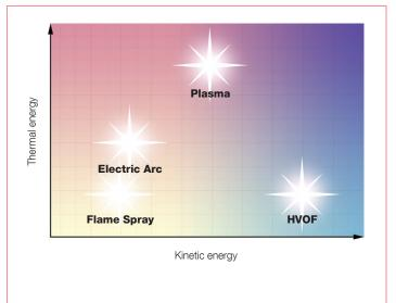
Figure 8 – Energy comparison of thermal spray processes
