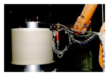
Figure 19 – Bearing shaft with a babbitt coating
