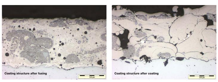
Figure 12 - Self-fluxing coating
