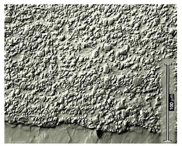
Figure 11 – HVOF spray coating of WC 12(CoCr)
