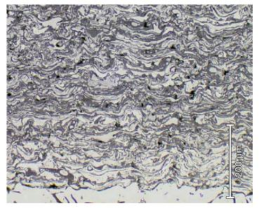
Figure 10 – Arc wire spray coating of X40 steel
