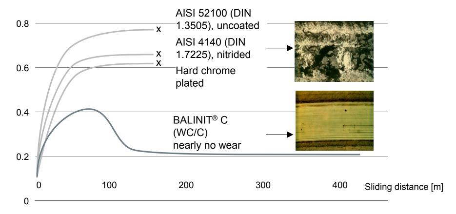
BALINIT® C (WC/C) shows under dry running condition the lowest friction and highest wear life time compared to conventional surface treatments.
