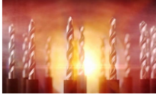
Drills getting coated in a PVD vacuum chamber
